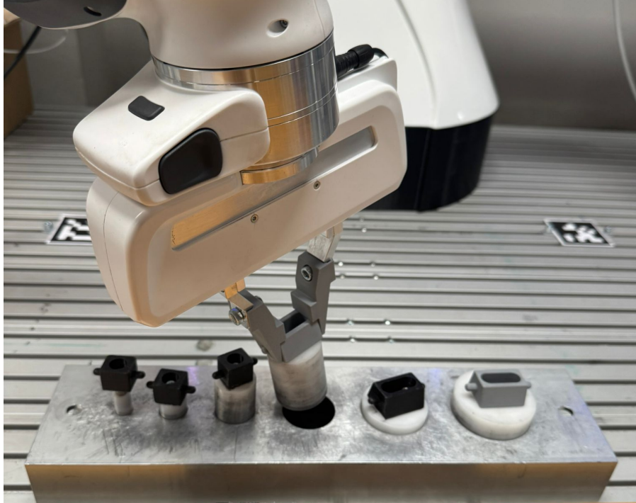
Figure 5.2: The robot aligns a cylindrical peg held in a parallel gripper with the fixture opening and performs a contact-rich peg-in-hole insertion under the different assistance modes.
